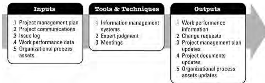
Figure 10-7. Control Communications: Inputs, Tools & Techniques, and Outputs
